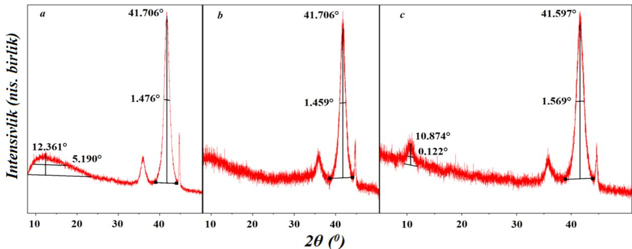
**8-rasm. (TiHfTa)CNning nurlantirilmagan (a) va  $2.5 \times 10^{17}$  el/sm<sup>2</sup> (b) hamda  $4.5 \times 10^{17}$  el/sm<sup>2</sup> (c) flyuenslarda nurlantirilgandagi rentgenogrammalari kesimi**
